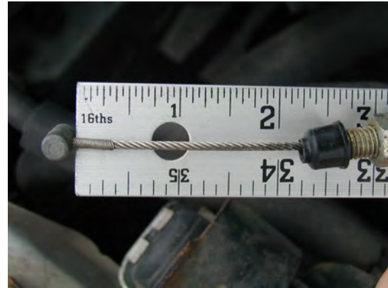
Illustration 4: Fully depressed throttle cable measurement
