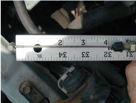
Illustration 3: Fully extended throttle cable measurement
