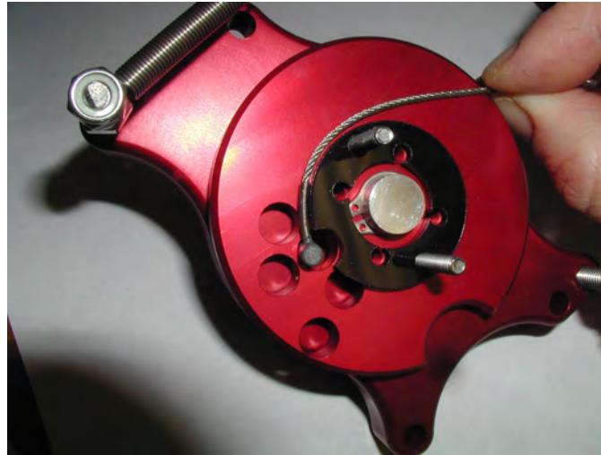
Illustration 5: Throttle cable barrel installation
